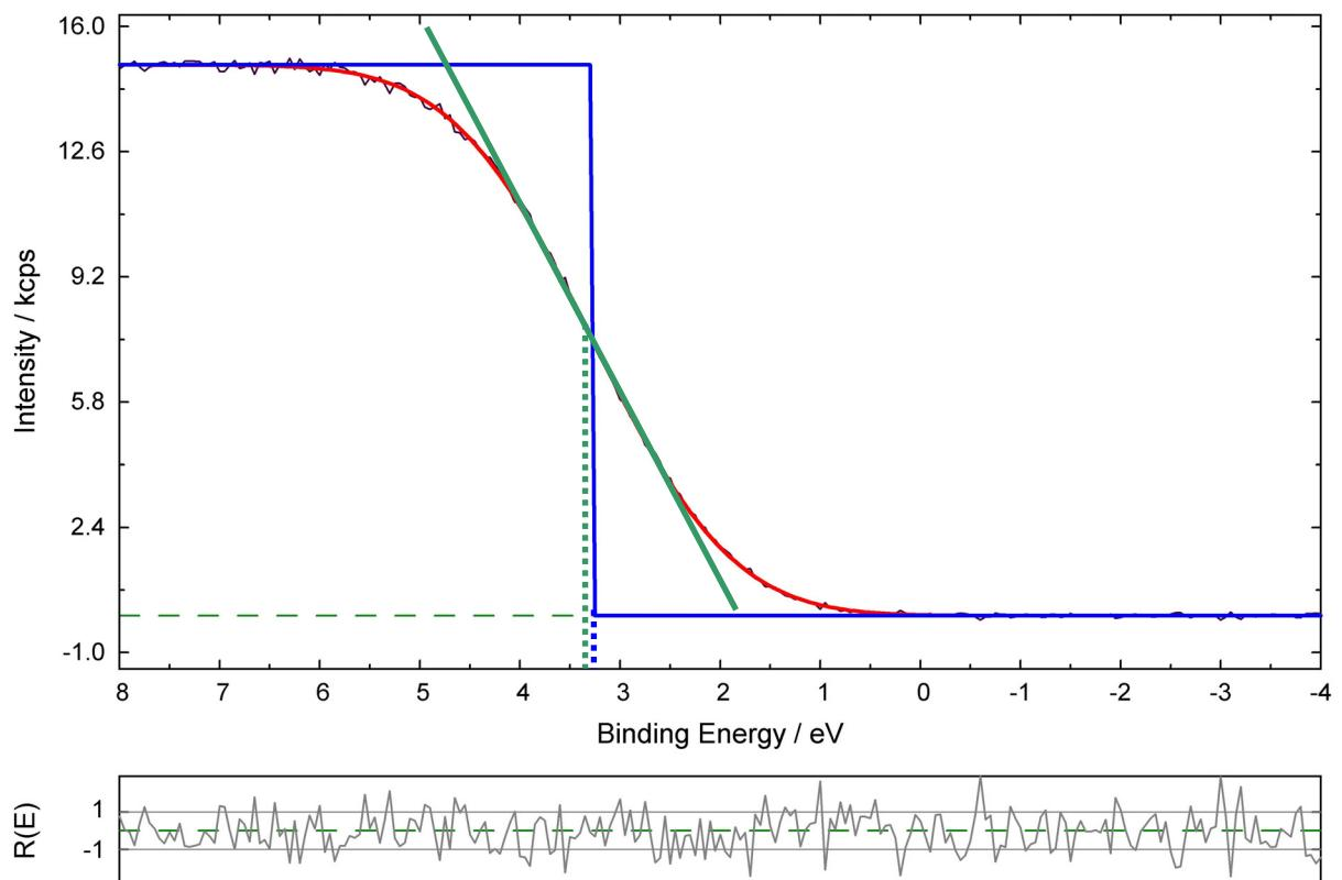
**Fig. 4.** Estimated Fermi edge, green: linear approximation,  $E_F = 3.35$  eV, blue: Theta function,  $E_F = 3.27$  eV, red: convolution function with Gaussian FWHM = 2.59 eV
