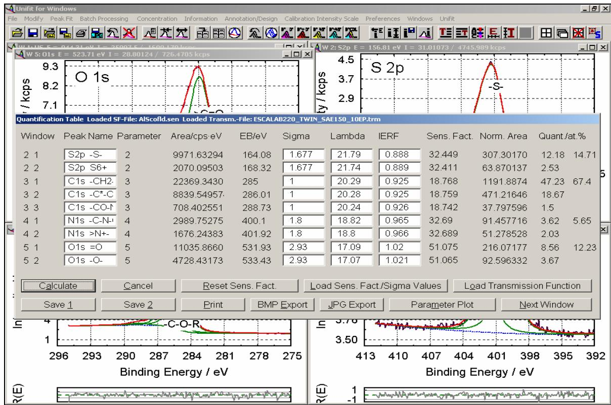
**Fig. 3.** Redesigned dialog of the quantification, the snap shot shows the example of sulphur, carbon, oxygen, and nitrogen using the sensitivity factor defined by the product of  $\sigma$ ,  $\lambda$  and the transmission function  $T(E)$  introduced by IERF.
